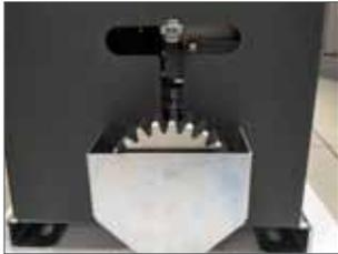
Mechanical limit switch with lever
