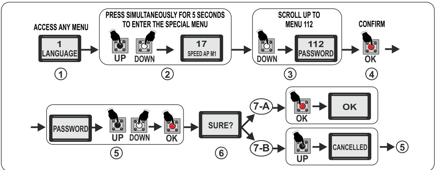
Once the password is activated, **the menus will only be shown but cannot be adjusted**; To unlock the control unit enter the correct password in the 112-PASSWORD Special Menu.
