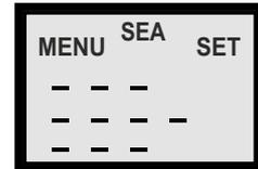
When a new or a just reset control unit is powered on, the display shows the software revision first then it shows the **INPUT STATUS** after 5 seconds. The latter will be the default display view when an already programmed unit is turned on
