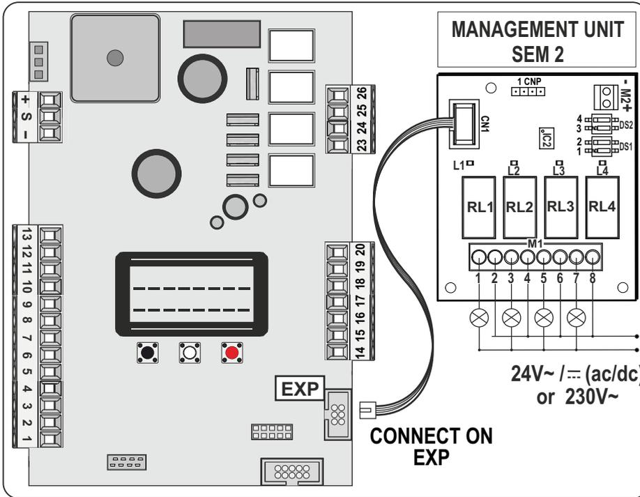
The «SEM 2» management unit can be connected through the **EXP** connector
