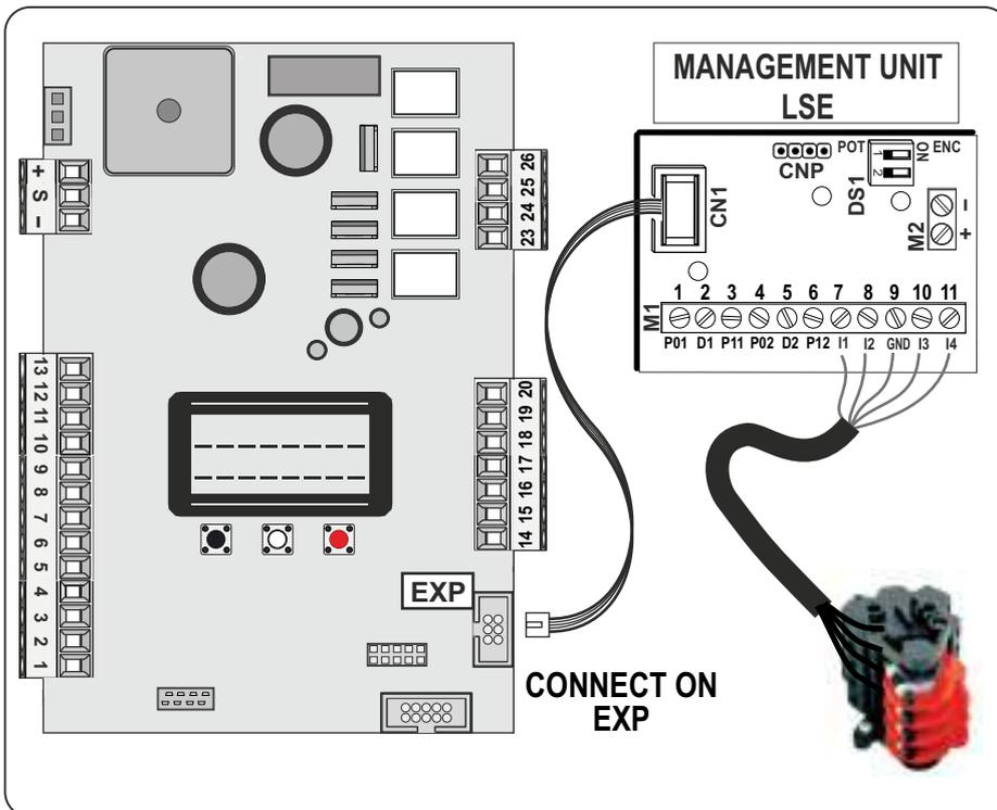
The «LSE» management unit can be connected through the **EXP** connector
