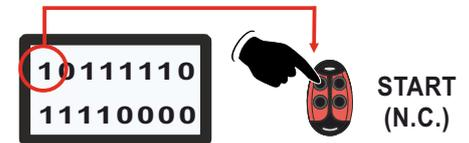
● Example: if you pass by the photocell, its input switches from normally closed to normally open
