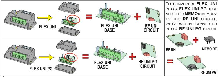
\* THE PLASTIC CASE OF THE **FLEX UNI** AND **FLEX UNI PG** RECEIVERS IS NOT CERTIFIED FOR THE «IP» PROTECTION DEGREE, THEREFORE THE MOUNTING IS ONLY RECOMMENDED IN CLOSED OR SHELTERED PLACES OR INSIDE THE JUNCTION BOXES;
