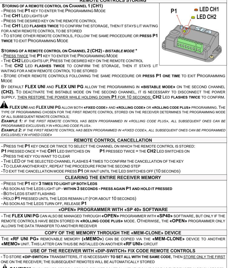
**A CAUTION!** IF YOU TRY TO STORE A SECOND REMOTE CONTROL WITH THE SAME CODE AS THE REMOTE ALREADY STORED, THIS LATTER WILL BE DELETED (4 FLASHES INDICATE THAT THE REMOTE CONTROL HAS BEEN DELETED); SIMILARLY, BE SURE TO SEND ONLY ONE IMPULSE WITH THE REMOTE CONTROL OTHERWISE THE SECOND IMPULSE CAN CANCEL THE FIRST ONE
