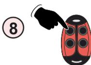
8 Once every control unit has been set up, power cycle the units, then send a «START» command to the «PRIMARY» control unit
